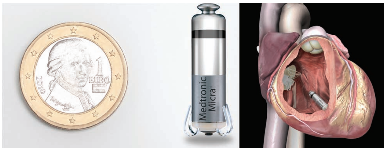
Fig 2. Medtronic Micra leadless pacemaker. A – compared in size to a one Euro coin; B – implanted. Reproduced with permission from Medtronic.
