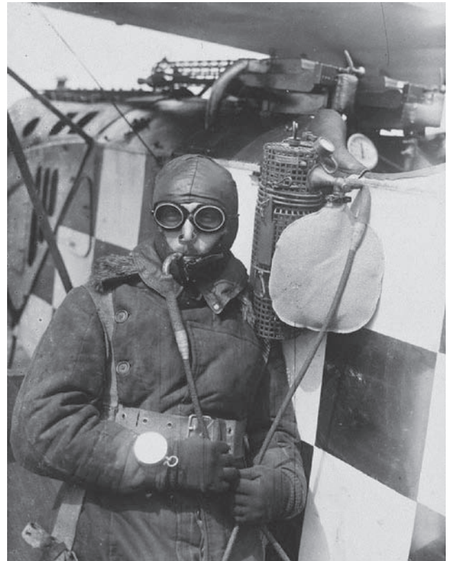
Fig 2. Continuous flow oxygen delivered by a tube held in the mouth. Reproduced with permission from the Farnborough Air Sciences Trust (FAST) archive.
