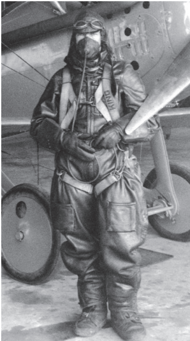
Fig 3. Continuous flow oxygen delivered by a tube inserted into a face mask. Reproduced with permission from the Farnborough Air Sciences Trust (FAST) archive.
